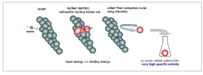
Figure 1. Production Molybdenum-99 using Molybdenum-98
