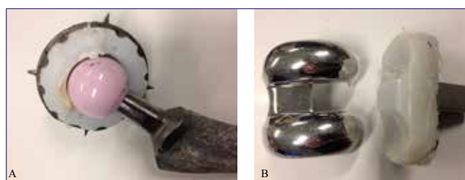
Figure 1. Pictures of retrievals showing wear of the bearing surfaces of total hip (A) and total knee (B) prosthesis, causing wear and small particle disease that can lead to aseptic loosening.
