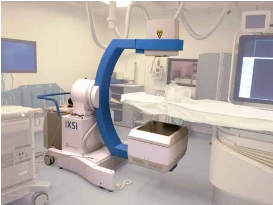
Figure 1. The developed hybrid c-arm scanner (named 'IXSI') that is placed in the intervention room of the UMC Utrecht.
